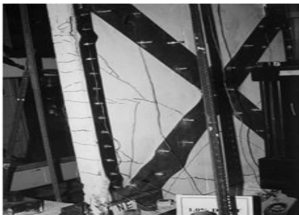
Figure 4 Retrofitted RC structure using steel bracings at 1.0 % drift
