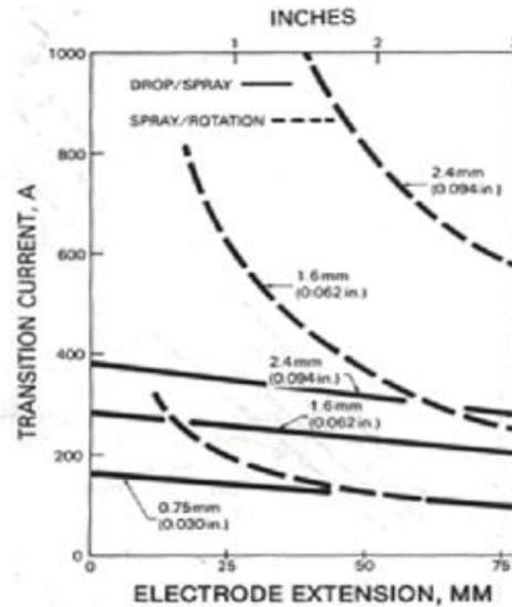
**Figure 10:** Effect of electrode extension and diameter on transition current [3]
