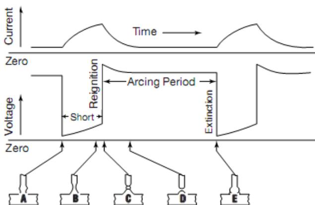
**Figure 5:** Oscillogram of short circuiting transfer [12]
