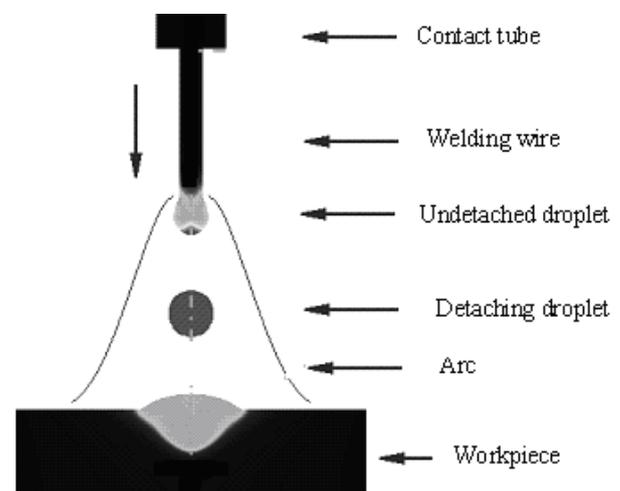
Figure 1: Metal transfer process in GMAW [2]
