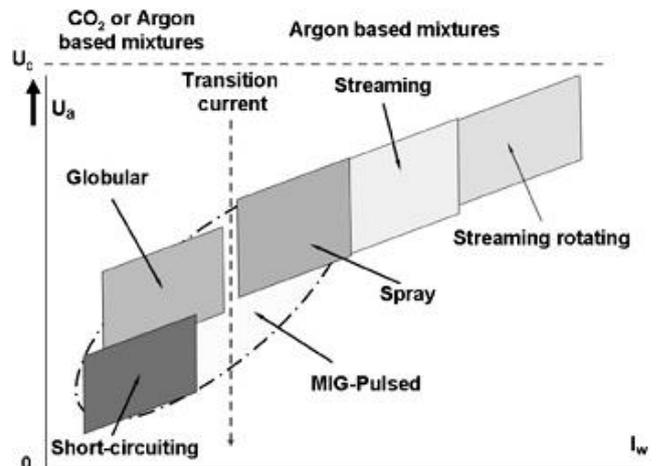
**Figure 7:** Arc voltage v/s welding current for various metal transfer modes [17]
