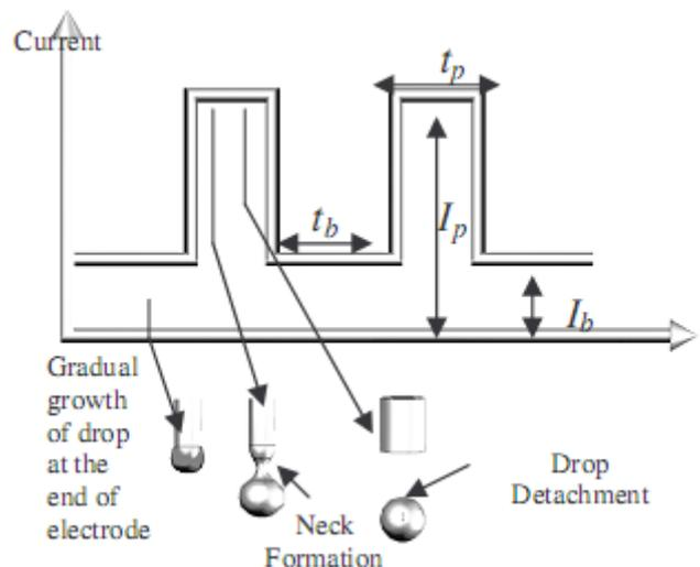
Figure 9: Pulsed current waveform [22]
