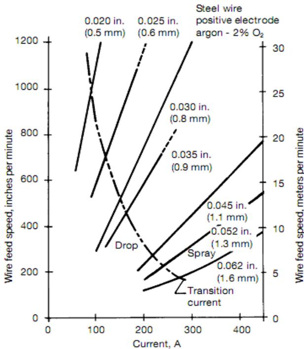
**Figure 6:** Burn-off curves of steel gas metal arc electrodes [19]
