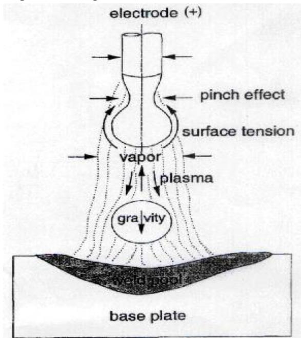
Figure 2: Forces acting on the drop [3]
