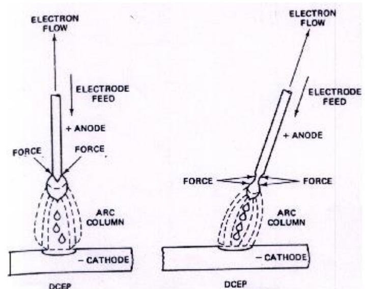
Figure 3. Electromagnetic forces on the drop [5]
