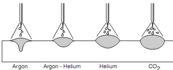
**Figure 11:** Bead contour and penetration patterns for various shielding gases [4]
