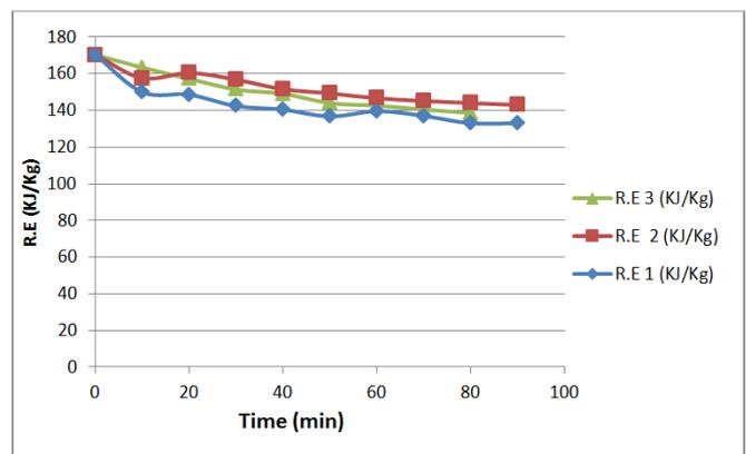
**Figure 3: Refrigerating effect vs time**
