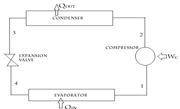
**Figure 1.** Vapour Compression Refrigeration Cycle
