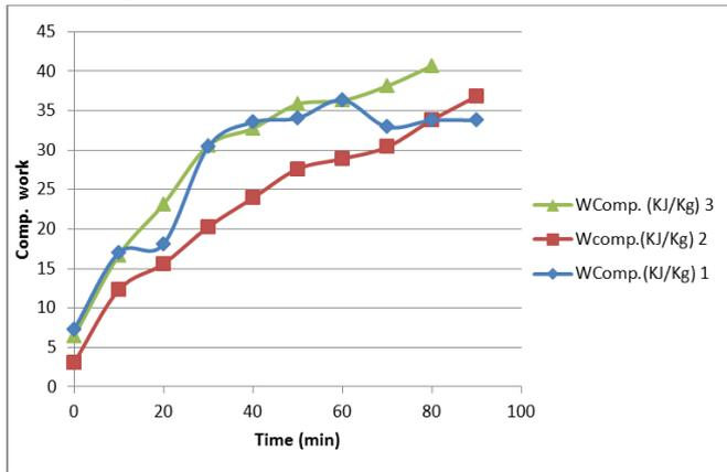
**Figure 5 : Compressor work vs time**
