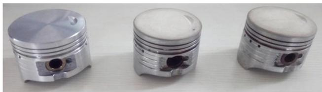
Figure 1. Uncoated and Coated piston
