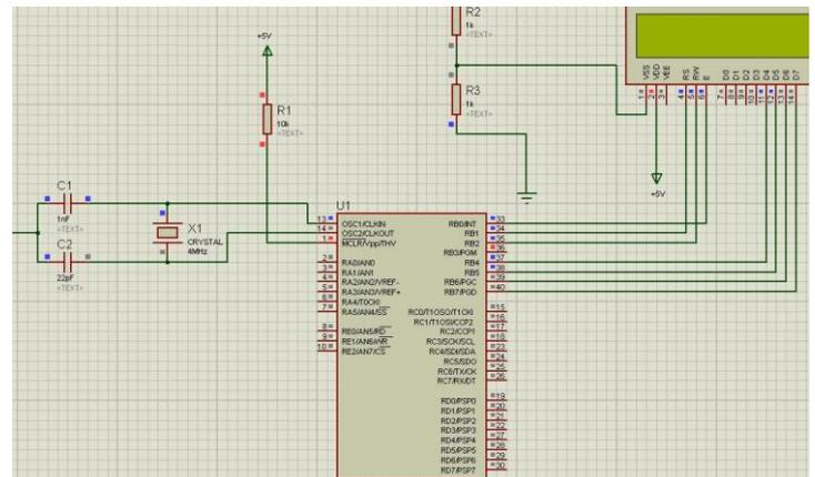
**Figure 5 Interfacing LCD with MC**
