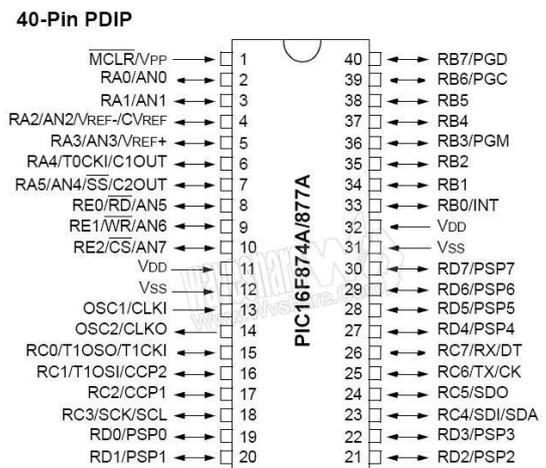
Figure 3. PIC16F877A Pin Diagram
