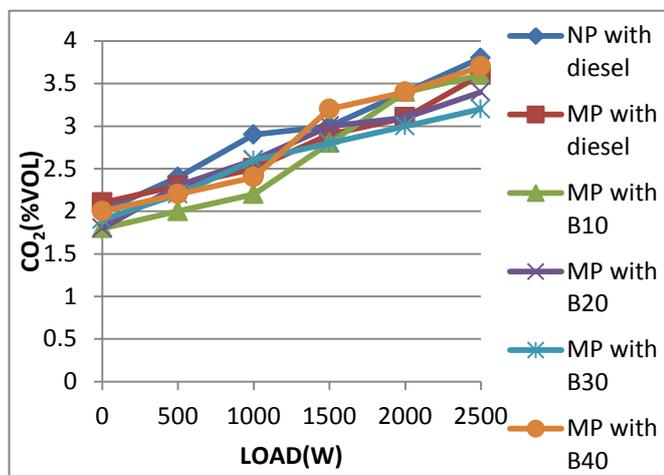
Figure 12. Load vs CO<sub>2</sub> Emissions
