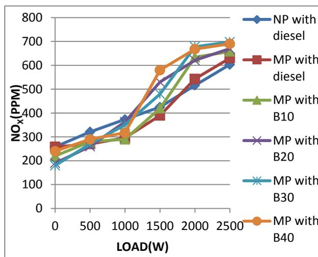
Figure 13. Load vs NO<sub>x</sub> Emissions
