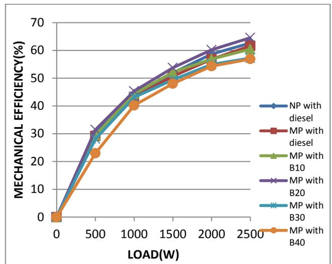
**Figure 8.** Load vs Mechanical Efficiency
