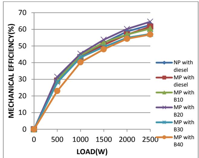
**Figure 8.** Load vs Mechanical Efficiency
