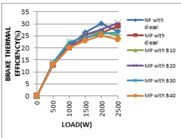
**Figure 9.** Load VS Brake Thermal Efficiency
