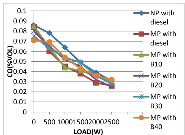
**Figure 10.** Load vs CO Emissions
