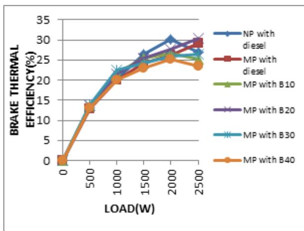
**Figure 9.** Load VS Brake Thermal Efficiency
