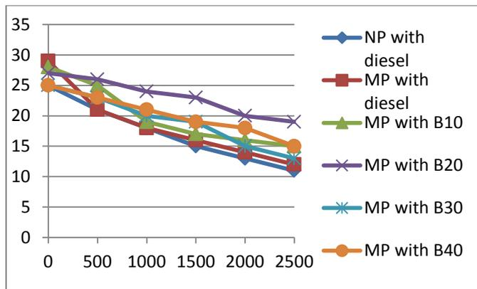
Figure 11. Load vs HC Emissions
