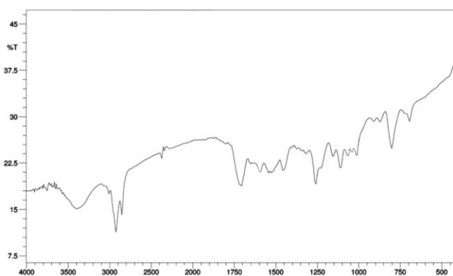
**Figure 1.** FT-IR spectrum of cardanol-based polyol
