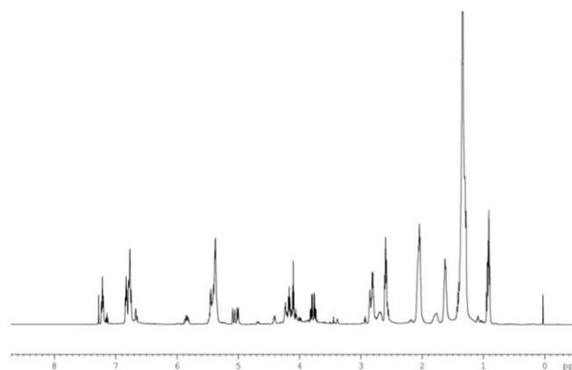
**Figure 2.**  $^1\text{H-NMR}$  spectrum of cardanol-based polyol
