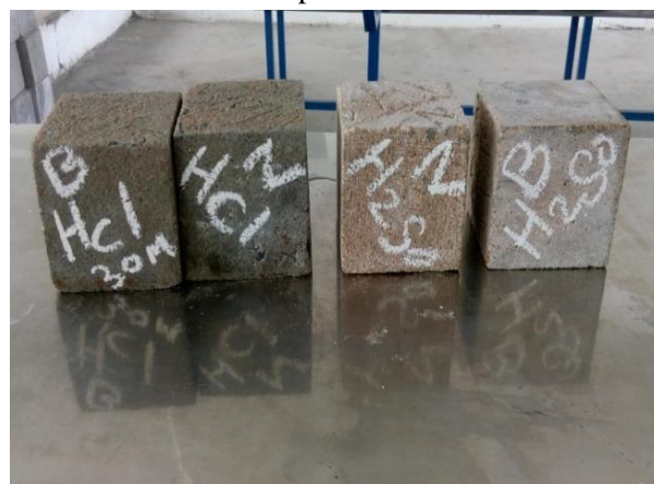
Fig.2. Specimens after immersed in HCL and H 2 SO 4 solution
