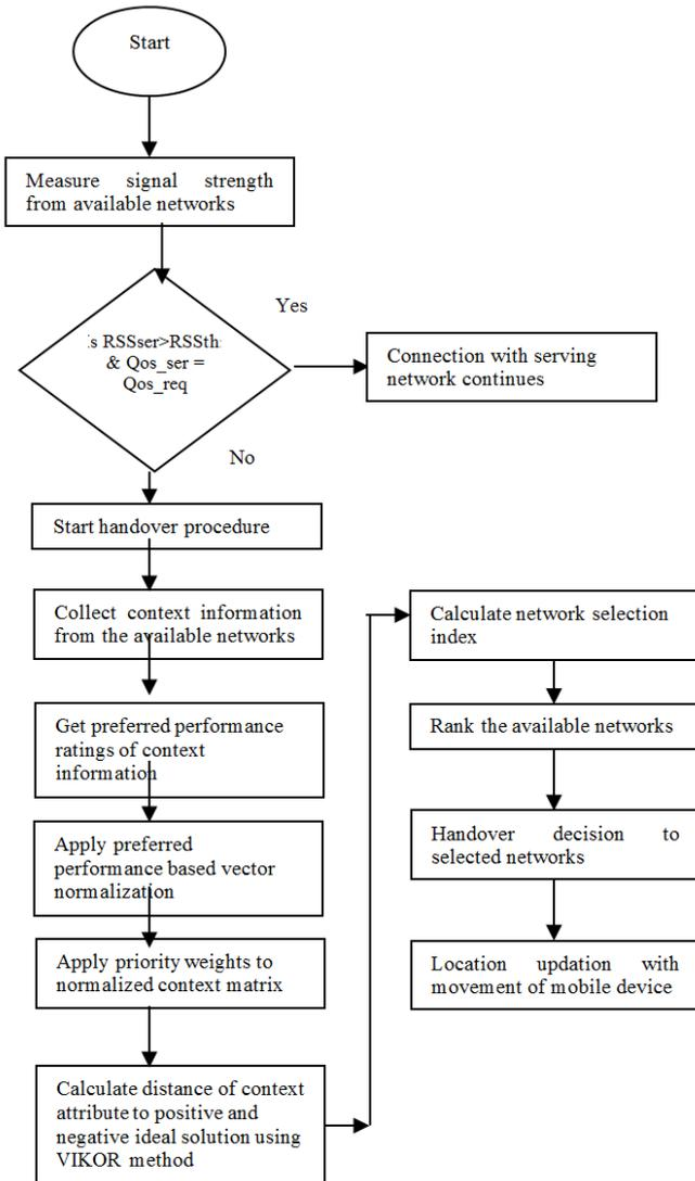
**Figure 1 :** Flow chart for mechanism of proposed method
