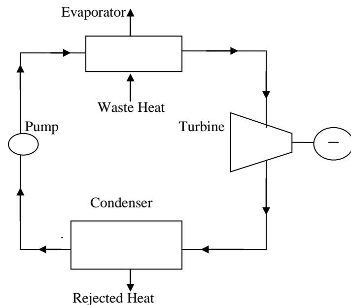
**Figure 1.** Schematic of Organic Rankine Cycle
