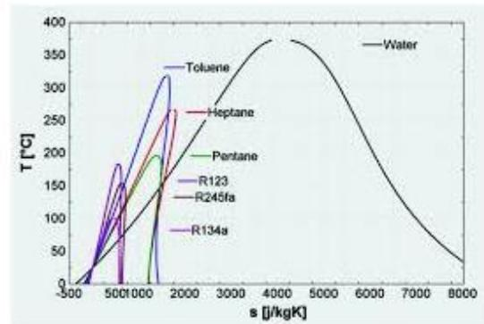
**Figure 2.** T-S diagram for different working fluids
