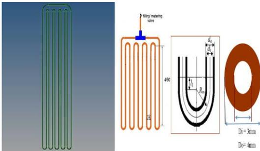
Figure 2. Closed loop pulsating heat pipe
