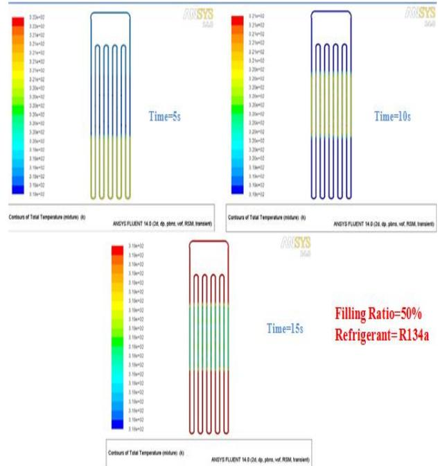
Figure 3. Contours of temperature variation in CLPHP
