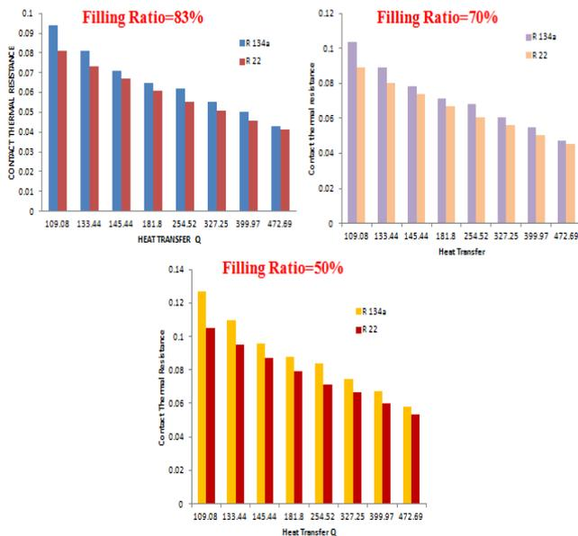
Figure 6. Contact thermal resistance of CLPHP
