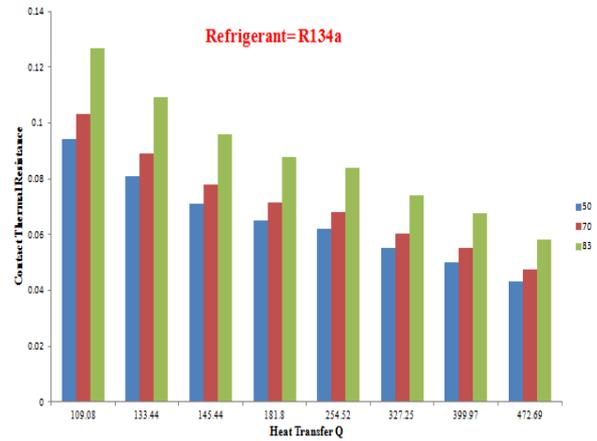
Figure 7. Variation of contact thermal resistance with filling ratio
