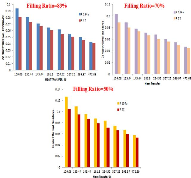
Figure 6. Contact thermal resistance of CLPHP
