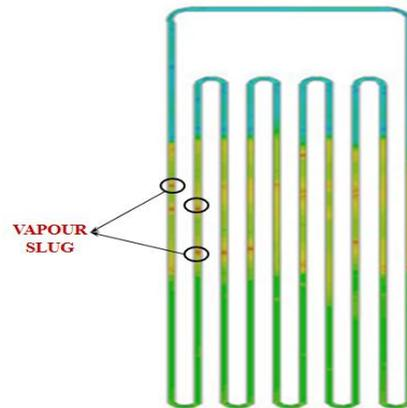
Figure 4. Vapour slug in CLPHP
