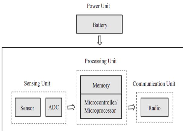
**Figure 2.** Sensor Node Structure
