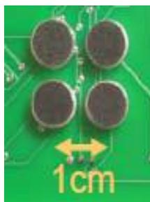
**Figure 2.2.** Acoustic sensor
