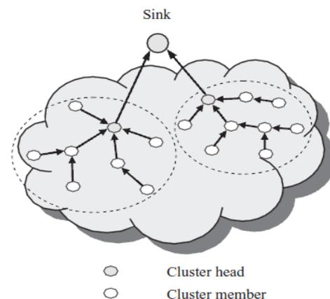
**Figure 3.** Hierarchical Architecture
