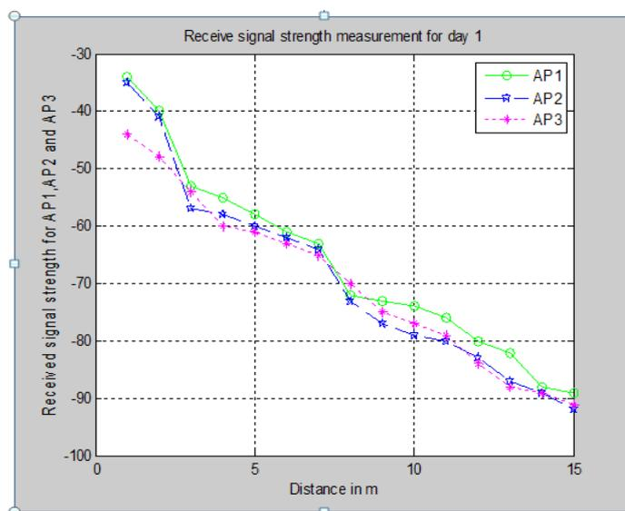
Figure 2: A graph of average received signal strength values (dBm) for the first month
