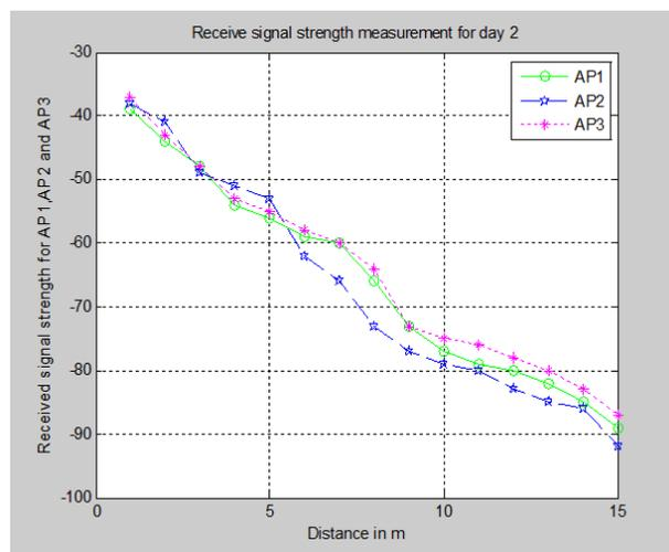
Figure 3: A graph of Average Received Signal Strength values (dBm) for the second month
