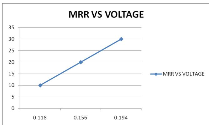
**Figure 10.** MRR Vs Voltage (3.1)
