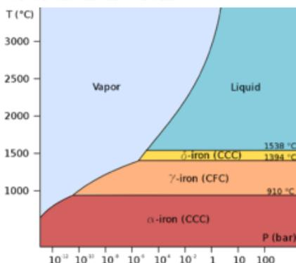
Figure 4. Low-Pressure Phase diagram of Iron
