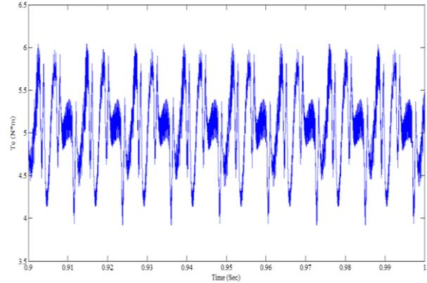
**Figure 13.** Torque waveform for Modified Miller Converter
