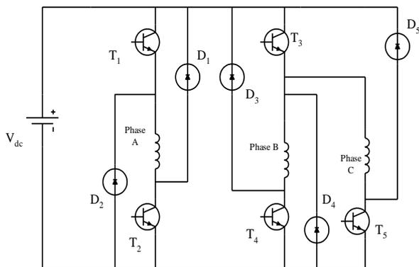
**Figure 4.** Modified Miller Converter
