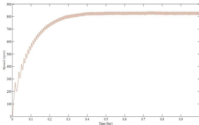
**Figure 8.** Speed waveform of Asymmetric Bridge Converter
