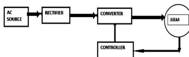
**Figure 5.1.** Block diagram of Switched Reluctance Motor
