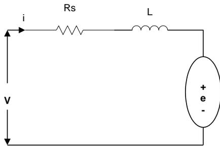
**Figure 1.** Equivalent circuit of SRM
