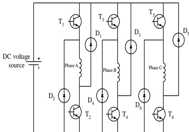
**Figure 2.** Asymmetric Bridge Converter
