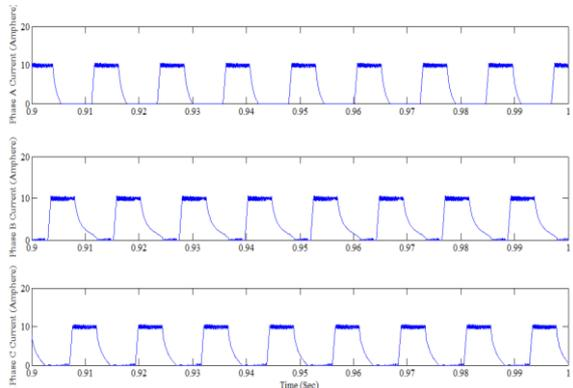
**Figure 12.** Phase current for Modified Miller Converter
