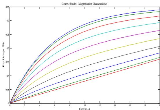
**Figure 5.2.** Magnetization Characteristics of SRM
