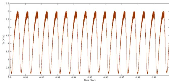
**Figure 7.** Torque waveform for Asymmetric Bridge Converter
