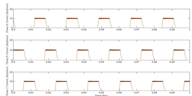
**Figure 6.** Phase current waveform for Asymmetric Bridge Converter
