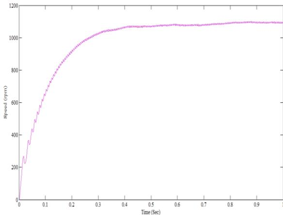
**Figure 11.** Speed waveform of Miller Converter
