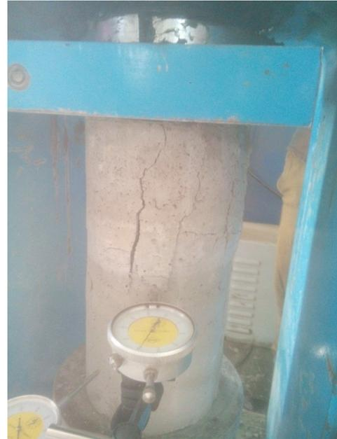
**Figure 2.** Failure mode for circular RCC Column specimens
