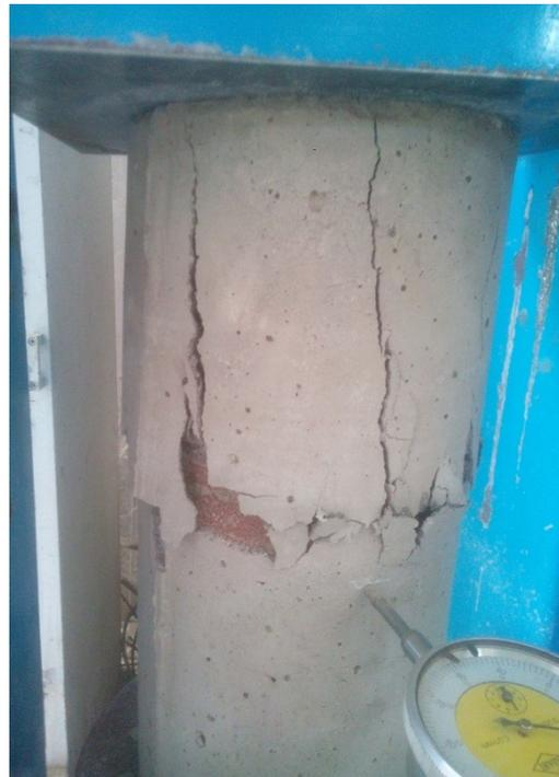
**Figure 3.** ultimate failure mode for RCC circular column
