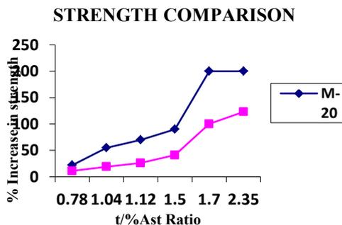
**Figure 1.** Graph showing strength comparisons for M-20 and M-25
