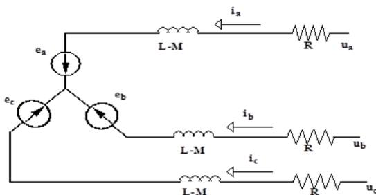
Figure 6. Equivalent circuit diagram of BLDC Motor
