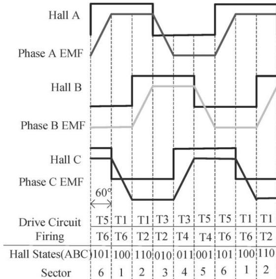
Figure 5. Back EMF BLDC motor phase
