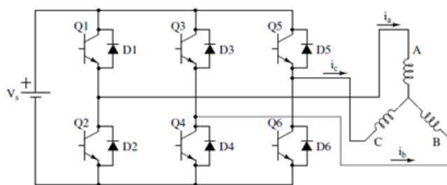
Figure 3. H-bridge inverter circuit
