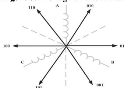
Figure 4. Six sectors of the BLDC motor voltage vector
