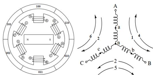
Figure 2. Y-connected BLDC motor construction
