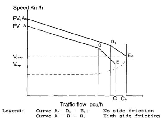
**Figure 1.** Impact of side friction on capacity
