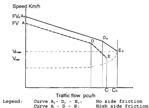
**Figure 1.** Impact of side friction on capacity
