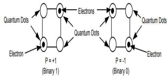
**Figure 1.** QCA Polarization cells with +1 for logic 1 and -1 for logic 0.
