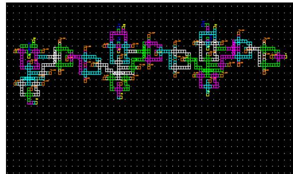
**Figure 14.** QCA layout for the Ripple carry adder.
