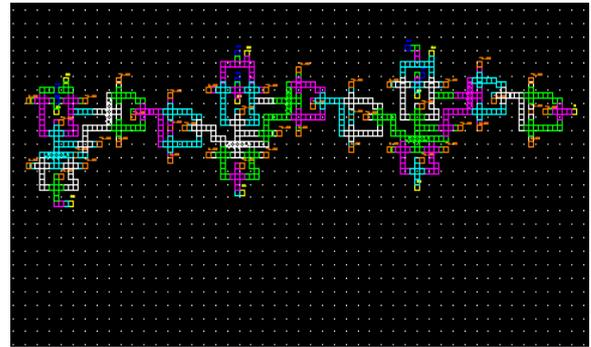
Figure 14. QCA layout for the Ripple carry adder.
