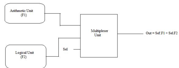
**Figure 11.** Integration of Arithmetic and Logical Unit
