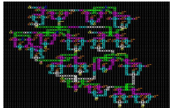
Figure 16. QCA layout for the Logic unit
