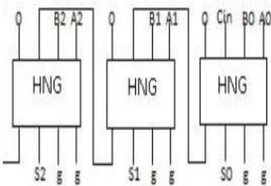
Figure 8. Ripple carry adder
