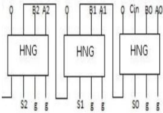
**Figure 8.** Ripple carry adder
