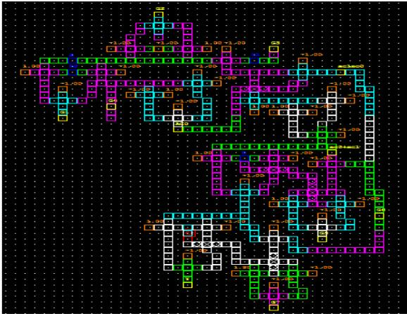
Figure 18. QCA layout for the Arithmetic unit.
