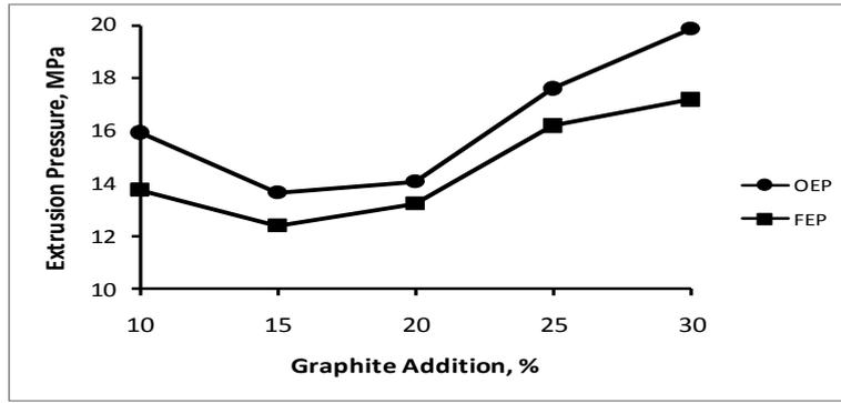
**Figure 1:** Variation in Extrusion Pressure versus Graphite Addition in the Lubricant
