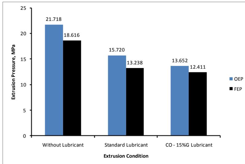
**Figure 2:** Comparison of OEP and FEP of the Three Lubrication Regime
