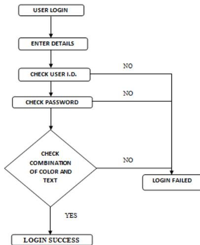
**Figure 11:** Architecture for the implemented module of Hybrid color and text.
