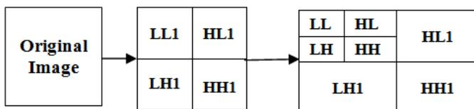
Figure 2: Decomposition at 3-level Wavelet
