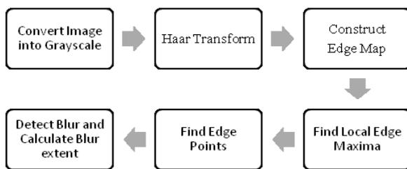
**Figure 3.** Blur Detection using Haar Transform [33]
