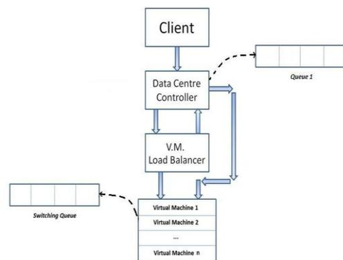
**Figure 4.** Priority Based Throttled Load Balancing Algorithm.
