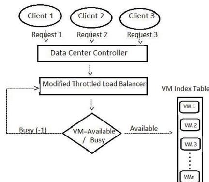
Figure 2. Flowchart of Modified Throttled Load Balancing Algorithm
