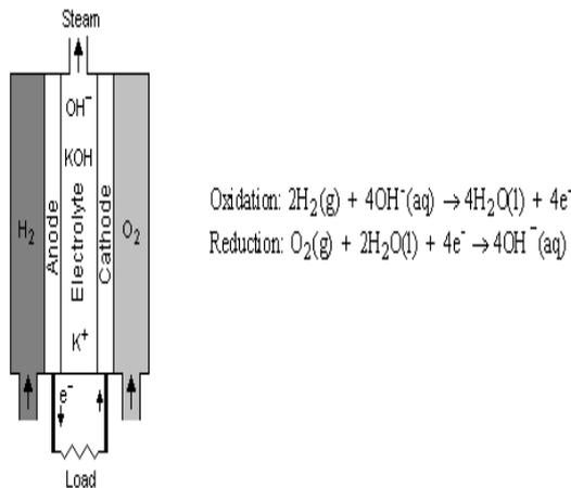
**Figure 1.** Alkaline fuel cell often uses hydrogen and oxygen as fuel
