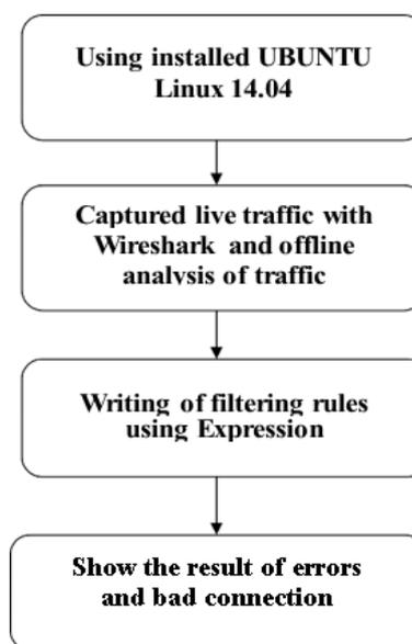
**Figure 1:** Implementation setup Diagram When capturing packets from a network interface, wireshark captures all of the packets coming and going
