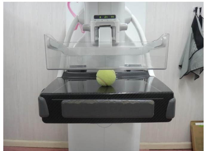
Figure 3: Set –up for measuring compression alignment
