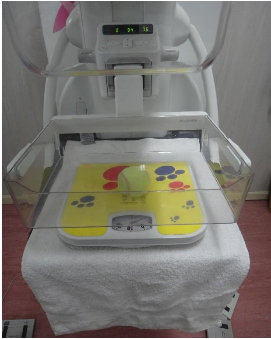
Figure 1: Set – up for measuring Compression force in Power and Manual Mode
