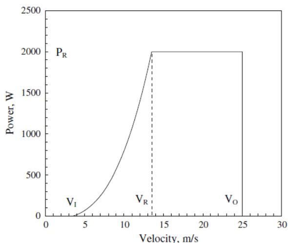
Fig.3 :Power curve of a 2 MW wind turbine
