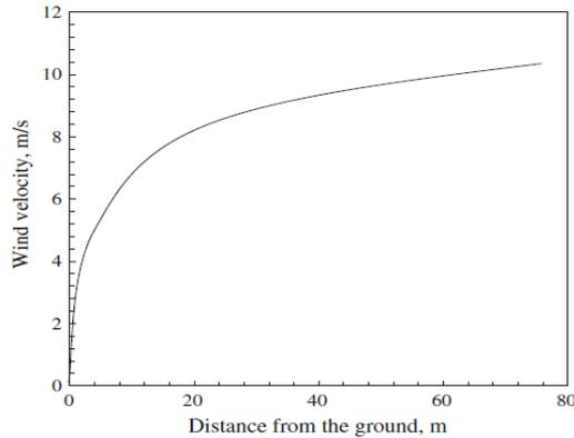
Figure 1: Variation of wind velocity with height
