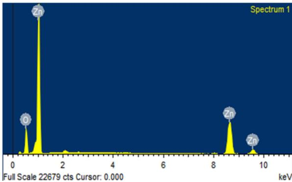
**Figure 3.** EDX Pattern of ZnO nanoparticles
