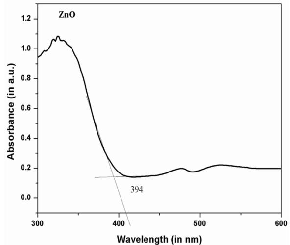
**Figure 4.** DRS image of ZnO nanoparticles.
