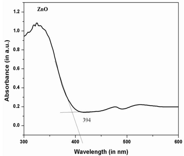
**Figure 4.** DRS image of ZnO nanoparticles.
