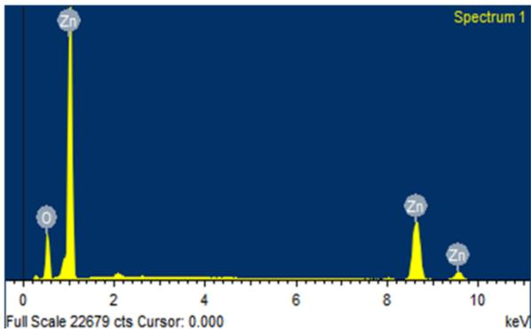
**Figure 3.** EDX Pattern of ZnO nanoparticles
