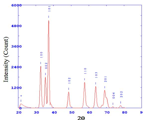
**Figure 1.** XRD Pattern of zinc oxide calcined at 500°C
