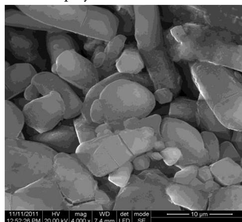
Figure 2. SEM image of the Ferrogel
