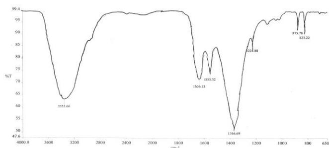
Figure-1. IR spectrum of poly (NTB-co-AM/MA)Ferrogel
