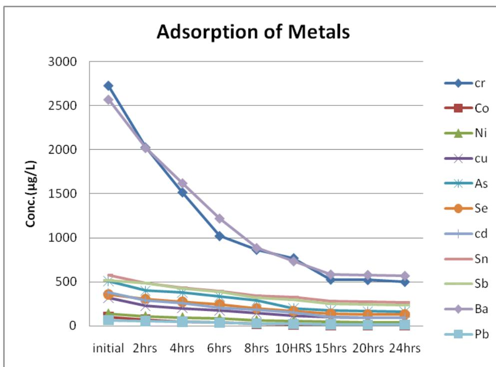
Figure-3. Removal of metal ions with time using Ferrogel
