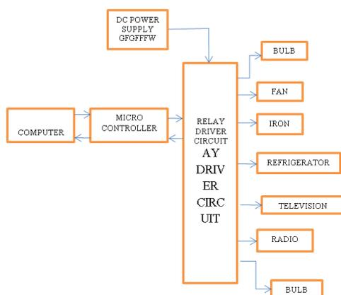
**Figure.2:** Block Diagram of the designed system
