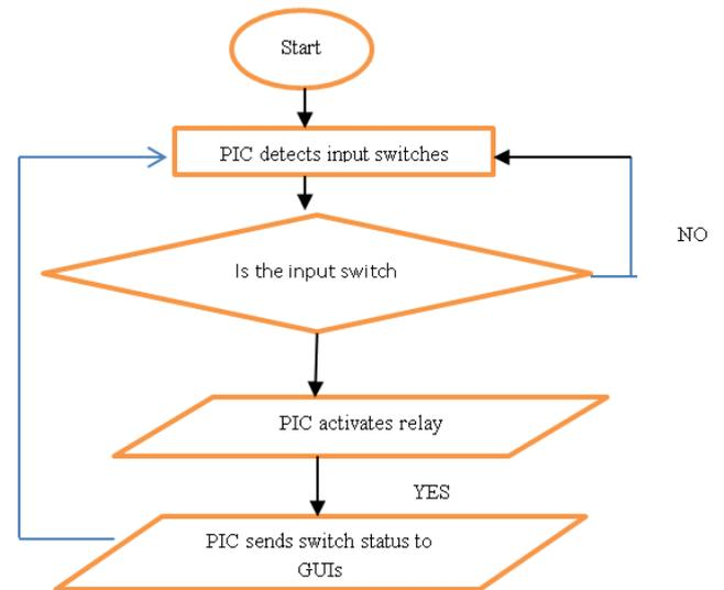
Figure 6: Flow chart showing PIC- GUI communication
