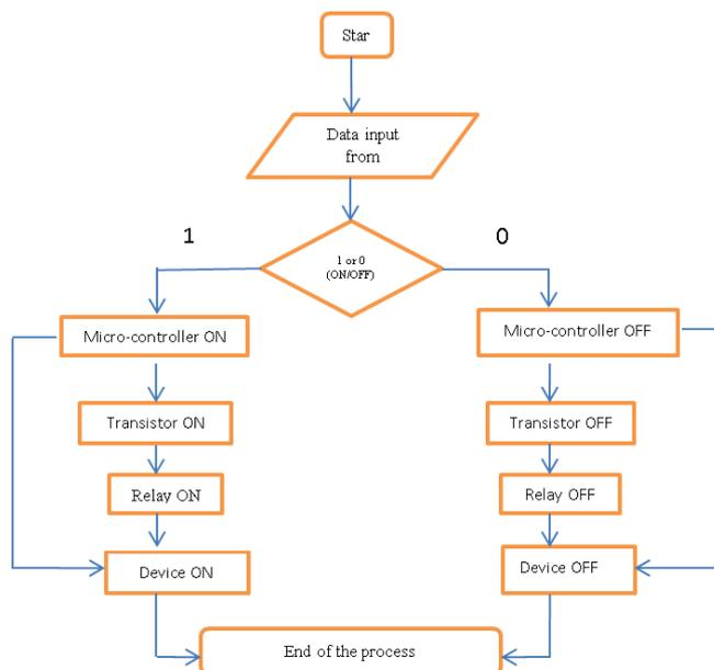
**Figure 7:** The flow chart of the designed system
