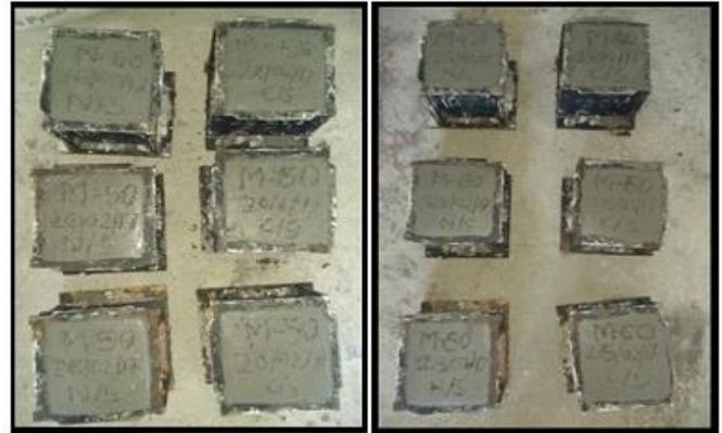
**Figure 12.** Casting of Cubes M50 and M60 grade of concrete.
