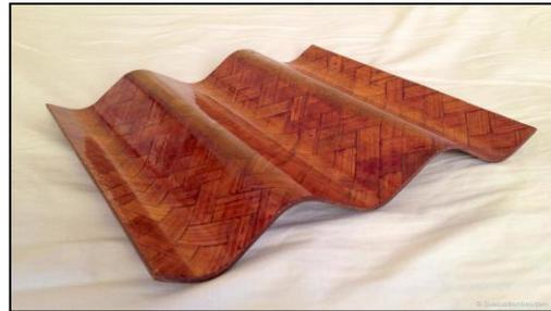
**Figure 9.** Bamboo matt corrugated roofing sheets
