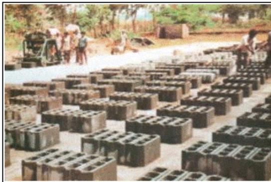
**Figure 5.** Bricks from Coal Washery Rejects
