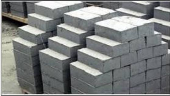
**Figure 4.** Fly ash-sand-lime bricks
