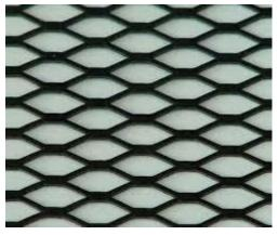
This mesh is formed by cutting a thin sheet of expanded metal to produce diamond shape openings. It is not as strong as woven mesh, but on cost to strength ratio, expanded metal has The advantage. This type of mesh reinforcement provides good impact resistance and crack control, but they are difficult to use in construction involving sharps curves.
