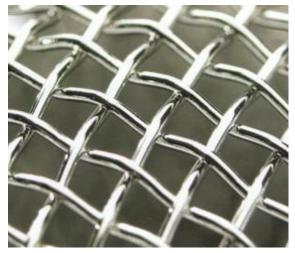
In this mesh, the wires are interwoven to form there required grid and the intersections are not welded. The wires in this type of mesh are not straight. They are bent in the shape of zigzag Lines and large angle of bending might cause cracks along the mesh However, the molding performance of this mesh is as good as the hexagonal and the welded wire mesh.
