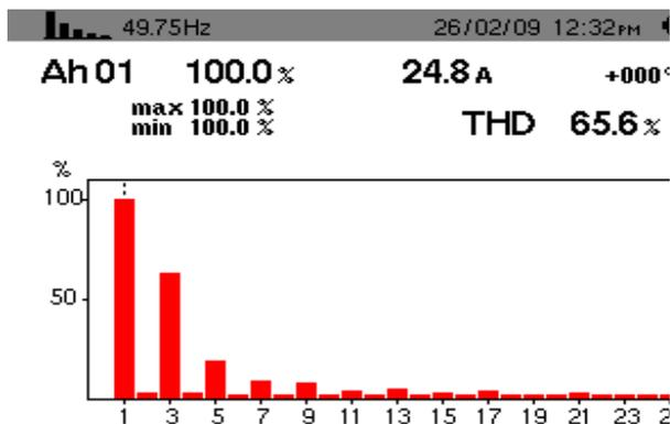
Figure 5a. FFT analysis of controlled rectifier
