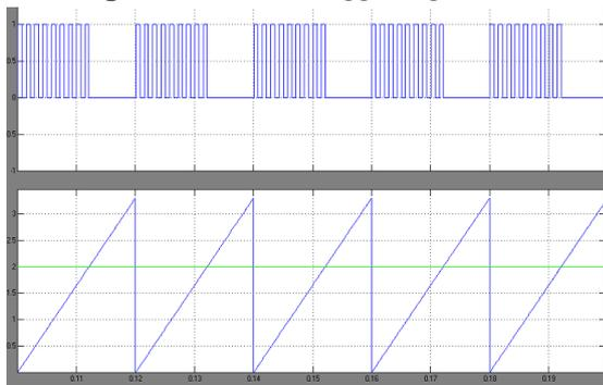
Figure 2(d). Gate triggering waveform
