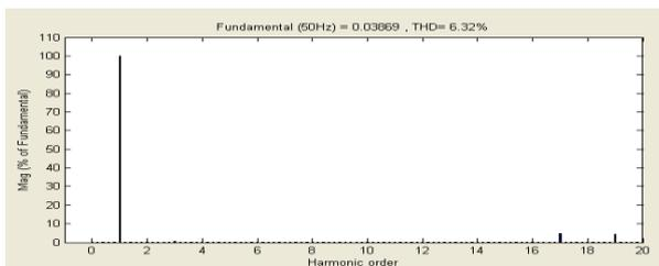
Figure 5. FFT analysis of PWM rectifier
