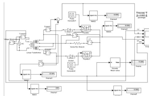
Figure 1(a). Controlled Rectifier circuit
