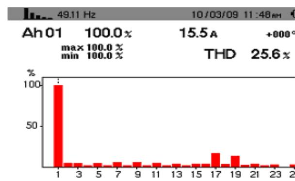
Figure 5b. FFT analysis of PWM rectifier
