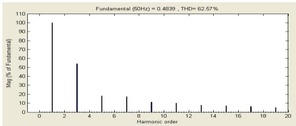
Figure 4. FFT analysis of controlled rectifier
