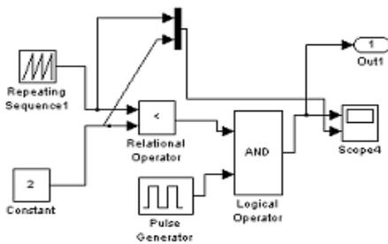
Figure 2(c). Gate triggering circuit
