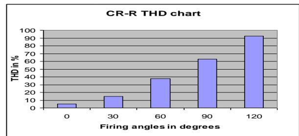
Figure 1(c). Firing angle
