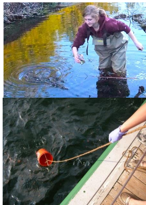
Figure 4: Grab sampling method used to collect water sample
