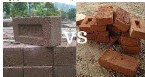
Figure 1. Flyash brick V/S Ordinary Clay brick
