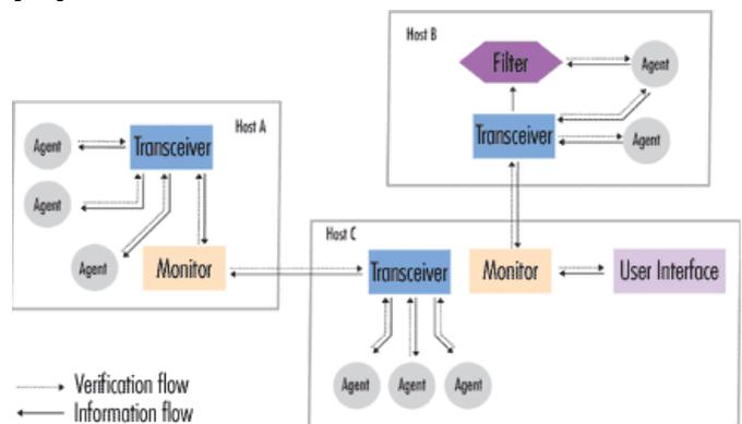
Figure 5. An AAFID compliant representation of an Intrusion Detection System employing autonomous agents [12]
