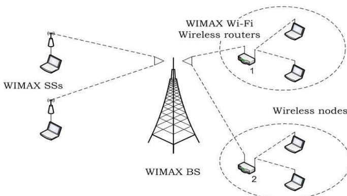
Fig. 2. WiMAX network architecture
