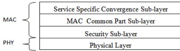
Fig. 1. Architecture of WiMAX layer
