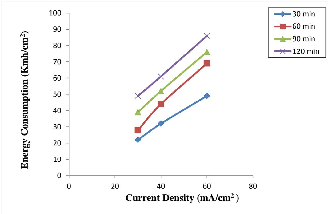
**Fig. 12.** Effect of current density on power consumption
