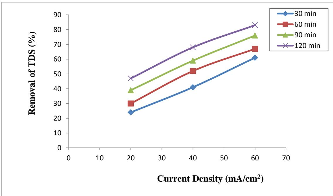
Fig. 4. Effect of current density on removal of total dissolved solids of Hindon water at 25.0 °C.
