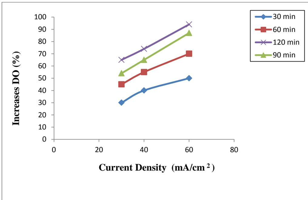
Fig. 7. Effect of current density on increasing of dissolved oxygen of Hindon water at 25.0°C.
