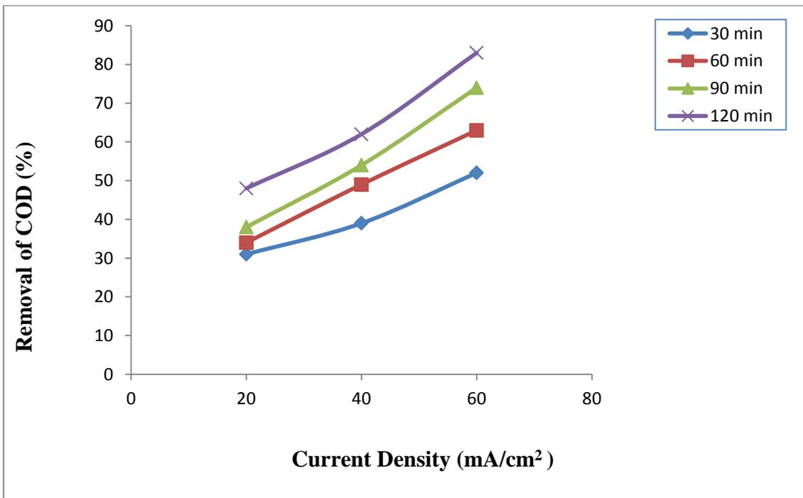
**Fig.2.** Effect of current density on removal of chemical oxygen demand of Hindon water at 25.0°C.
