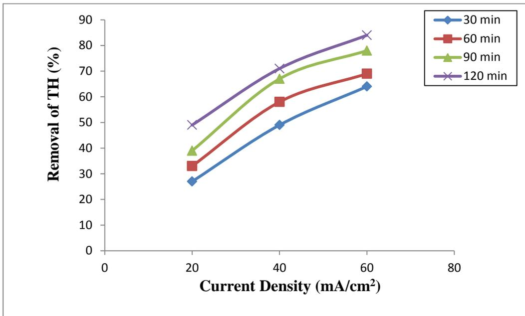
Fig. 5. Effect of current density on removal of total hardness of Hindon water at 25.0°C.
