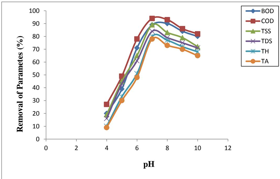
**Fig. 10.** Effect of pH on selected various parameters of Hindon water at 25.0 °C.
