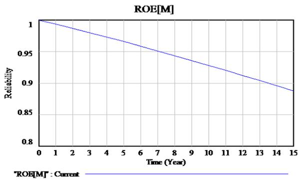
**Figure 5:** Graph showing reliability of overall evaporator including all components with time
