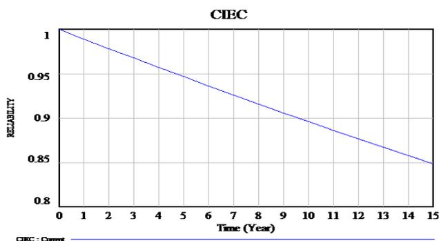
Figure 2: Reliability of evaporative coil regarding to its choking with time
