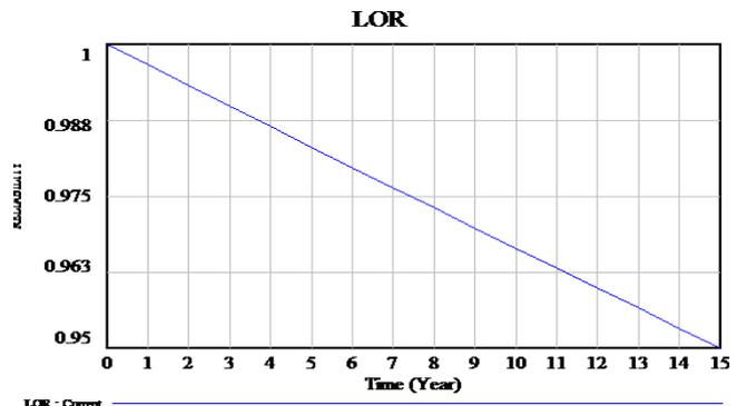
Figure 3 : Reliability variation of evaporator regarding to its leakage of refrigerant with time
