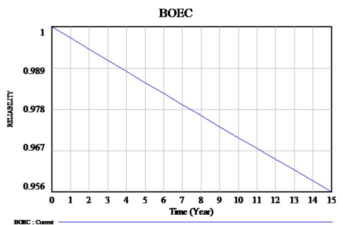
Figure 4 : Reliability of evaporator regarding to blockage in evaporative coil with time.
