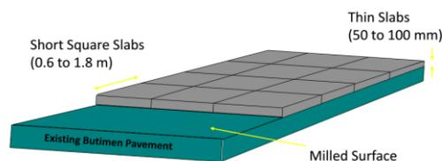
**Figure 2.** 3D view of Ultra-Thin White Topping
