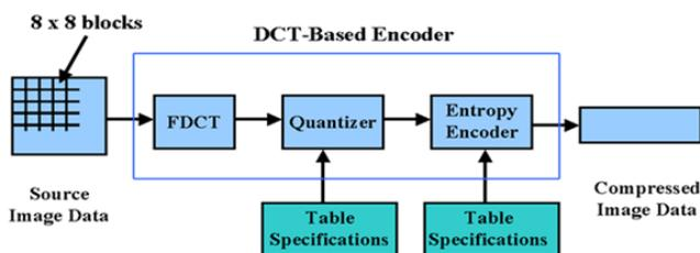
Figure 3.1. DCT-Based Encoder Processing Steps
