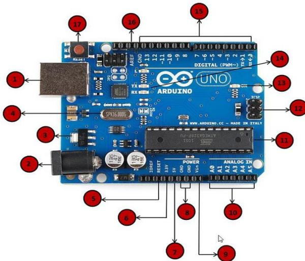
1. **Power USB:**Arduino board can be powered by using the USB cable from your computer. All you need to do is connect the USB cable to the USB connection (1).
