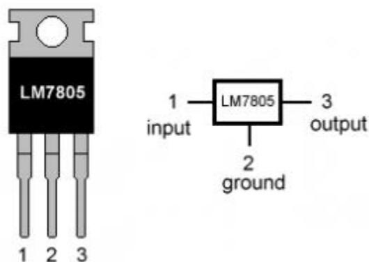
Figure 2. LM7805 Pinout Diagram
