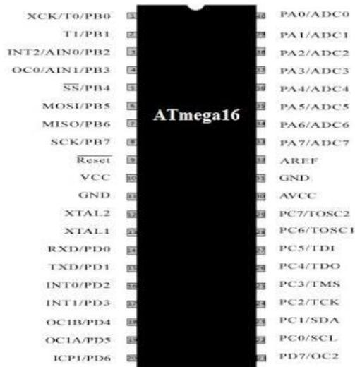
**Figure 3.** AVR atmega 16 microcontroller
