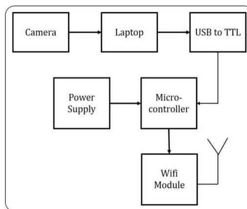
**Figure 3.** Transmitter module
