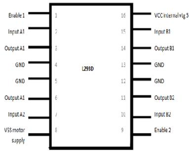
**Figure 4.** Pin configuration of L293D Motor driver IC
