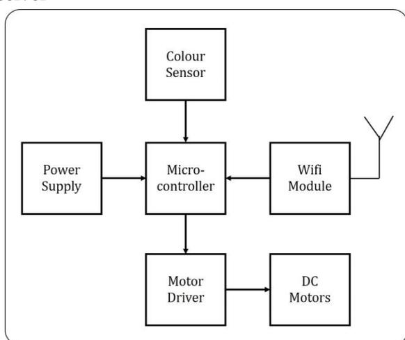
**Figure 2.** Receiver module
