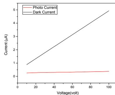
**Figure 2.** Photoconductivity of silver nitrate doped Zinc potassium phosphate hexahydrate
