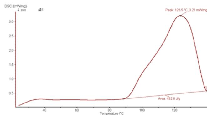
**Figure 3.** Differential scanning calorimetry (DSC) of silver nitrate doped Zinc potassium phosphate hexahydrate
