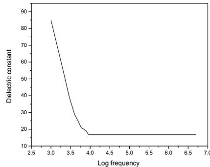
**Figure 5.** Dielectric constant of silver nitrate doped Zinc potassium phosphate hexahydrate single crystal
