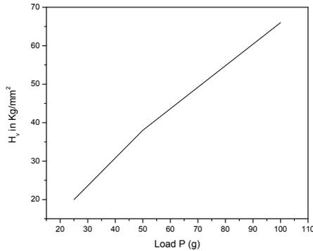
**Figure 4.** Microhardness of silver nitrate doped Zinc potassium phosphate hexahydrate single crystal
