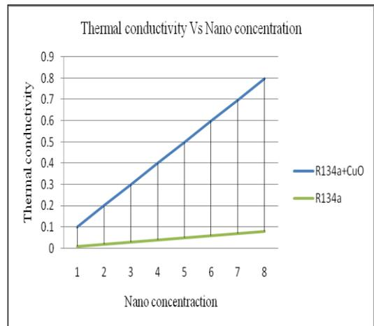
**Figure 1.** Effect of nano concentration on thermal conductivity
