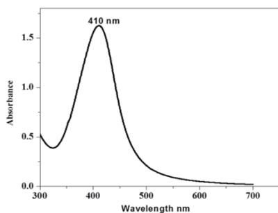
**Figure 1.** UV-Visible absorbance and IR spectrum of synthesized AgNPs from aqueous leaf extract of *Coleus vettiveroids*
