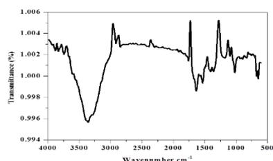
**Figure 2.** FTIR spectrum of synthesized AgNPs.
