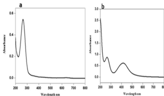
**Figure 4.** UV-Visible absorbance spectra of prepared (a) soap (b) soap impregnated with AgNPs.
