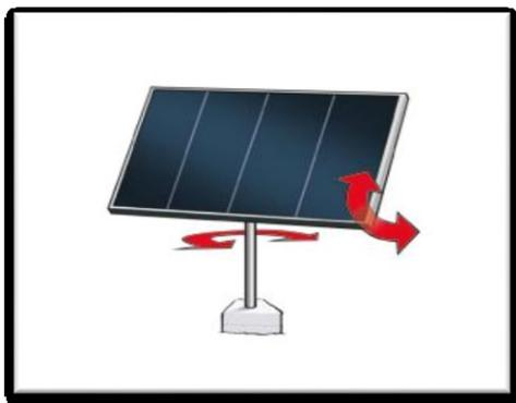
Figure 2. Dual Axis Tracking
