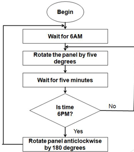
Figure 4. Flow chart Uniform Tracking method
