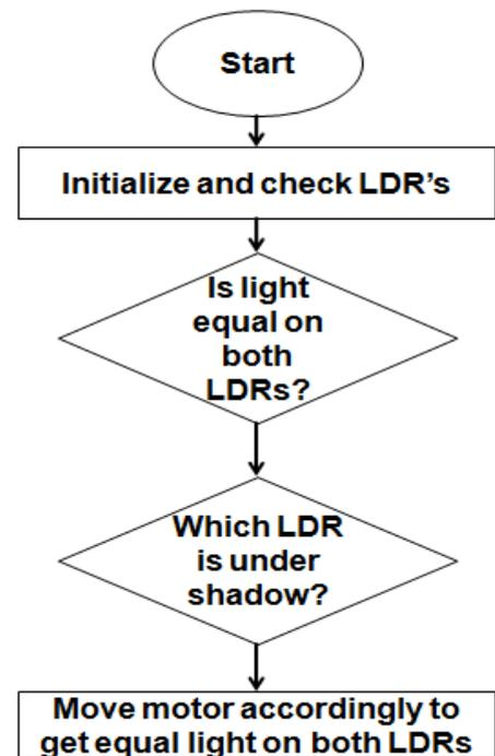
Figure 3. flow chart LDR Based Tracking method
