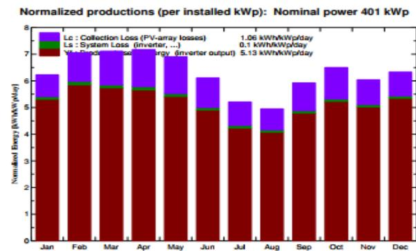
**Figure 11.** Normalized production for single axis tracking system
