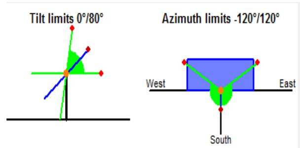
**Figure 10.** Tracking dual axis
