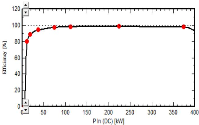
**Figure 7.** Efficiency curve of 374 KW Inverter
