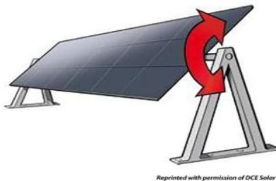
Figure 1. Single Axis Tracking
