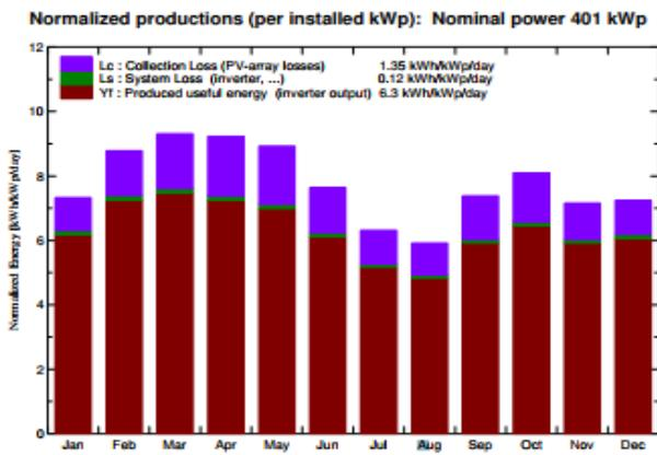
**Figure 13.** Normalized production for dual axis tracking system.
