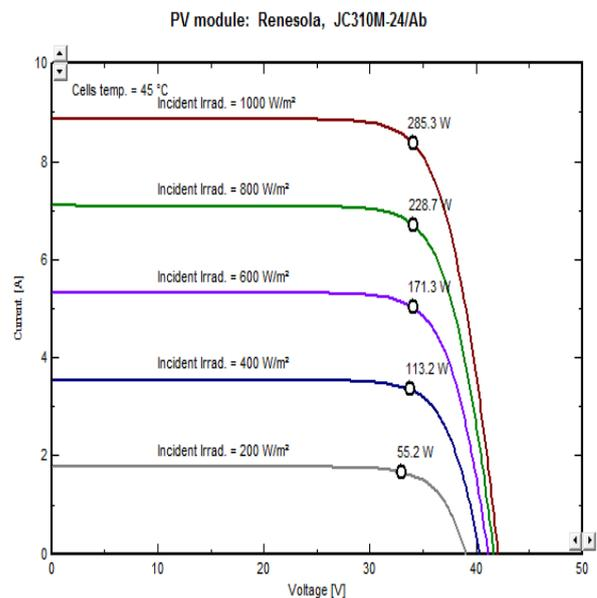
**Figure 3.** V-I Characteristics of PV panel
