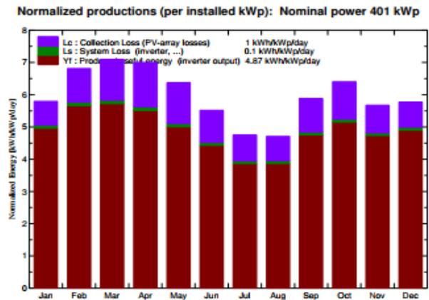
**Figure 11.** Normalized production for fixed solar system
