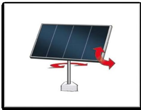
Figure 2. Dual Axis Tracking
